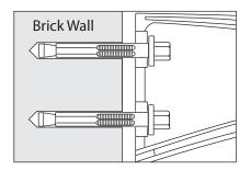
Insert assembled anchor into hole, so that washer or head is flush with materials to be fastened. \*DO NOT unscrew the head. Insert it as is. If it is stiff, use rubber hammer to insert.
