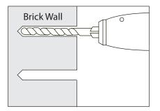
Use a bit whose diameter equals the anchor diameter. Determine proper size bit for anchor used. Drill hole to any depth exceeding minimum embedment. Clean hole.
