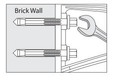
3. Expand anchor by tightening nut or head 2 to 3 turns.
